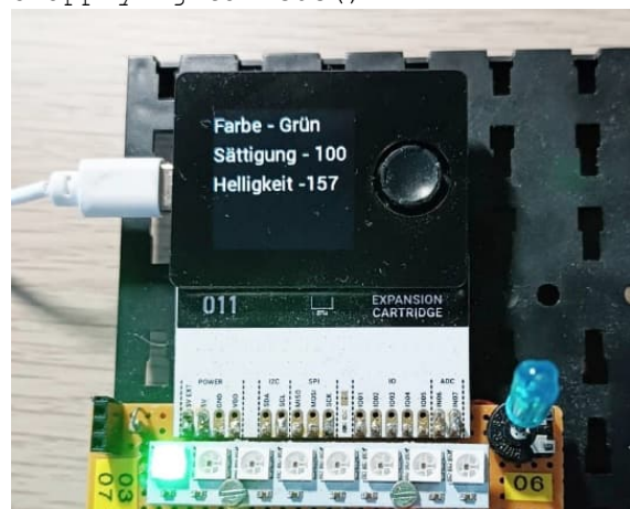
Abb. 11: RGB-LED (WS2812) an der Oxocard
