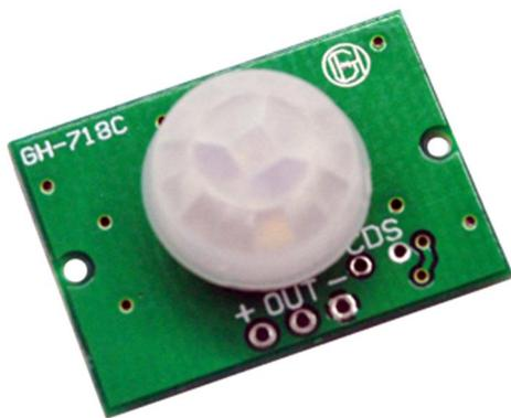
Abb. 6: PIR-Sensor GH-718C
