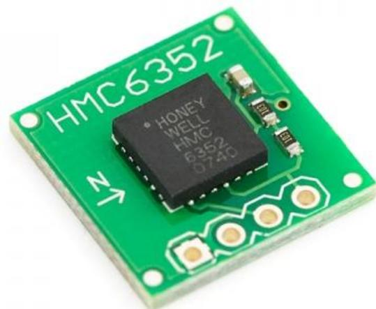
Abb. 1: Kompass-Sensor HMC6352 [3]
